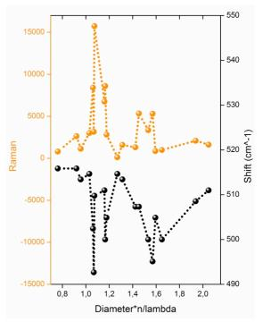
Fig. 2. Dependence of maximum light-induced heating of silicon nanoparticles on their diameter (n is a refractive index of silicon, *lambda* is a wavelength of a He-Ne laser). Temperature is reflected in the Raman shift [3]; while the intensity of the Raman signal
