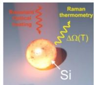
Fig. 1. Schematic illustration of strong optical heating and Raman thermometry of silicon nanoparticle.
